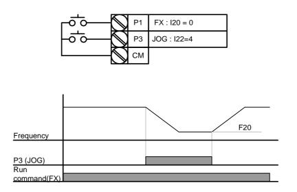
Jog operation overrides all other operations except Dwell operation. Therefore, if Jog frequency command is entered in the middle of Multi-Step, Up-Down or 3-wire operation, operation is executed at Jog frequency.
